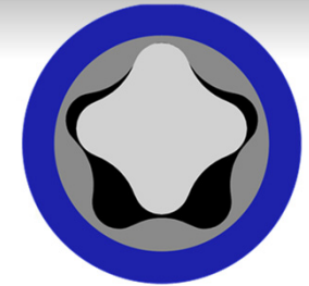
RECOMMENDED ROTOR / STATOR FIT
